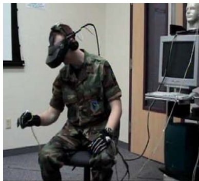
Figure 2. Concept for GOSE immersive system with improved HMD and data gloves.
